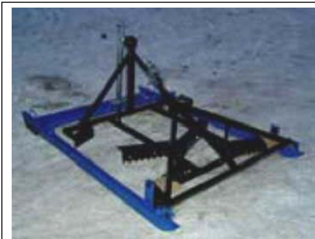
The adjustable teeth on this Renovating Leveller can cut into hard trail surfaces, or, when raised, allow packing and levelling of light, fluffy snow.
