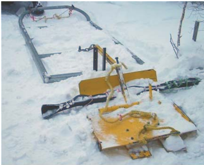
One Pass Grooming: the Norman Wells Ski Club groomer drags a 'bed-frame' type leveller and tracksetter in tandem. The snowmobile does the packing.
