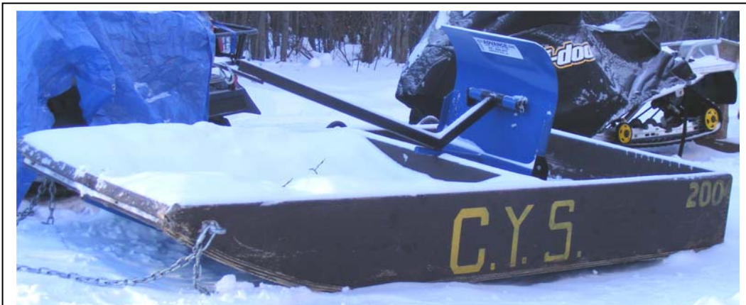
In Nahanni Butte, a compaction-type pan is filled with snow and pulled behind a snowmobile to pack 5 km of double-wide classic trails.
