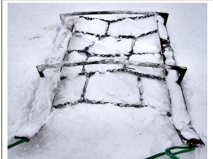
*K'atl'odeeche First Nation ski trails are levelled and renovated with a home-made chain drag. Chains are welded to old 'Cat' blade runners and tightened with turnbuckles.*
